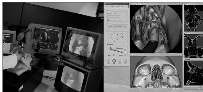
Figure 4. Virtual simulator of nasosinus endoscopic surgery (ES3). Computer screen image of this software to the side. Note the possibility of changing virtually the tweezers, other tools, and dissection images.
