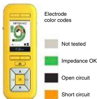
Figure 2 Information available for the remote assistant after evaluating the impedance and information on the electrode status.
